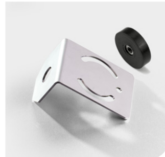
WA-Mount-NF-3 Antenna Mount Stainless steel wall mounting bracket with 16.5 mm mounting hole for antennas. Mounting on metallic surfaces via enclosed magnets. The holes for wall mounting can also be used for cable ties.
